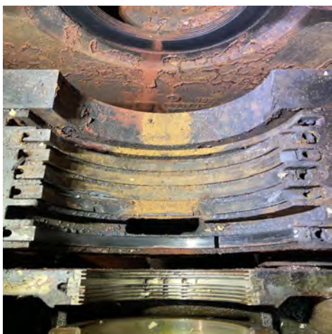
Exhaust End Carbon Seal Rings, As Found
