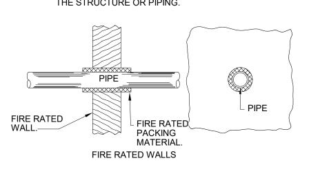
2 PIPE THRU WALL DETAIL NTS
