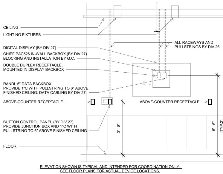
A3 TYPICAL AUDIO/VISUAL ELEVATION - DIGITAL DISPLAY 1/2" = 1'-0"
