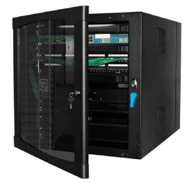
30" DEEP - WALL MOUNTED CABINET Similar to CUBE-IT Wall-Mount Cabinet; Gen 3; 48"H x 24"W x 30"D (1220 mm x 610 mm x 760 mm); 26U; #12-24 Tapped Rails; Tempered Glass Door; Black
