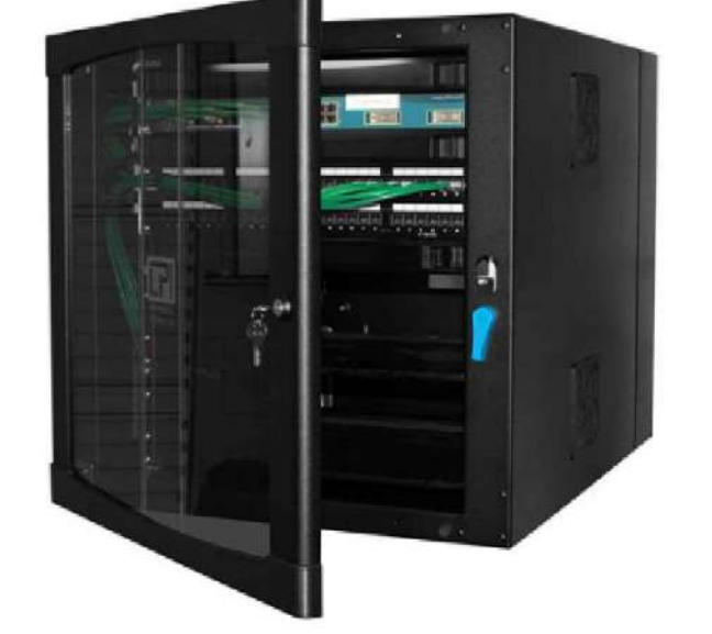
30" DEEP - WALL MOUNTED CABINET Similar To CUBE-IT Wall-Mount Cabinet; Gen 3; 48"H x 24"W x 30"D (1220 mm x 610 mm x 760 mm); 26U; #12-24 Tapped Rails; Tempered Glass Door; Black
