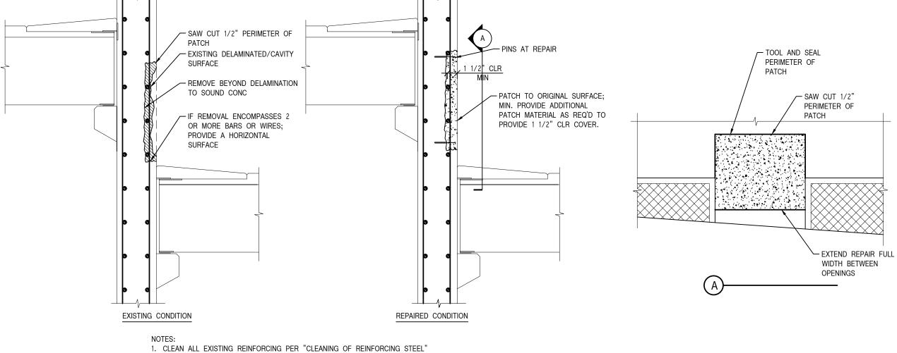
2. EPOXY COAT ALL EXISTING REINFORCING AFTER CLEANING. 3. FOR BID: LINEAR FEET OF PERIMETER TOOL AND SEAL SHALL BE 3 TIMES THE REPAIR QUANTITY.
