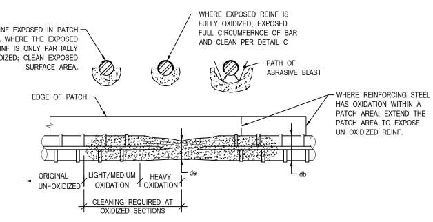
1. IF REINFORCING HAS LOST MORE THAN 20% OF THE CROSS SECTIONAL AREA (de = 0.9x db) REPAIR THE REINFORCING STEEL BE REPLACING OR ADDING ADDITIONAL REINFORCING. ALL NEW/REPLACMENT REINFORCING MUST BE TENSION LAP SPLICED WITH FULL SECTION OF EXISTING REINF. 2. REMOVE ALL OXIDATION AND SCALE FROM THE REINFORCING AND EMBEDS WITH OIL-FREE ABRASIVE BLASTING. 3. EPOXY COAT ALL EXPOSED REINFORCING AFTER IT IS CLEANED FREE OF OXIDATION.
