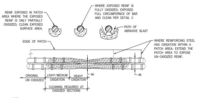
1. IF REINFORCING HAS LOST MORE THAN 20% OF THE CROSS SECTIONAL AREA (de = 0.9x db) REPAIR THE REINFORCING STEEL BE REPLACING OR ADDING ADDITIONAL REINFORCING. ALL NEW/REPLACMENT REINFORCING MUST BE TENSION LAP SPLICED WITH FULL SECTION OF EXISTING REINF. 2. REMOVE ALL OXIDATION AND SCALE FROM THE REINFORCING AND EMBEDS WITH OIL-FREE ABRASIVE BLASTING.
